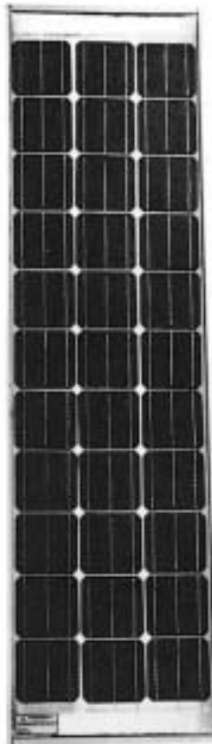
40-W high-density solar module: 100-mm × 100-mm square cells are used to provide maximum power in a minimum of space. The 33 series-cell module provides a strong 12-V battery charging current for a wide range of temperatures (−40°C to 60°C).
