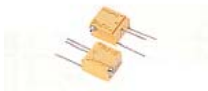
(c) Cermet multiturn trimming potentiometer
