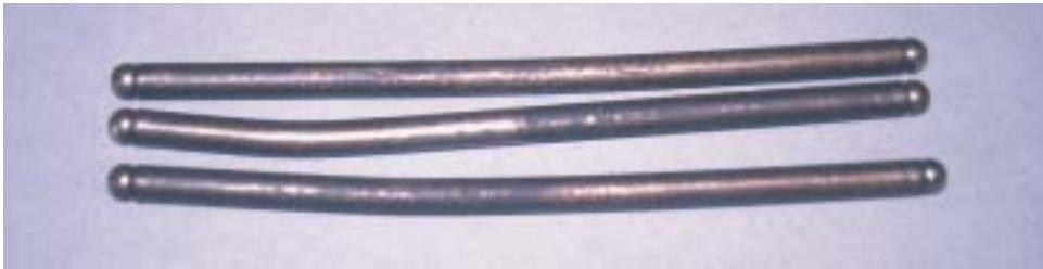
Figure 9–19 When the timing chain broke, it caused the camshaft to go out-of-time, which allowed the pistons and valves to collide on this interference engine. This may also bend the pushrods. Valve-to-piston contact will not occur on freewheeling engines.
