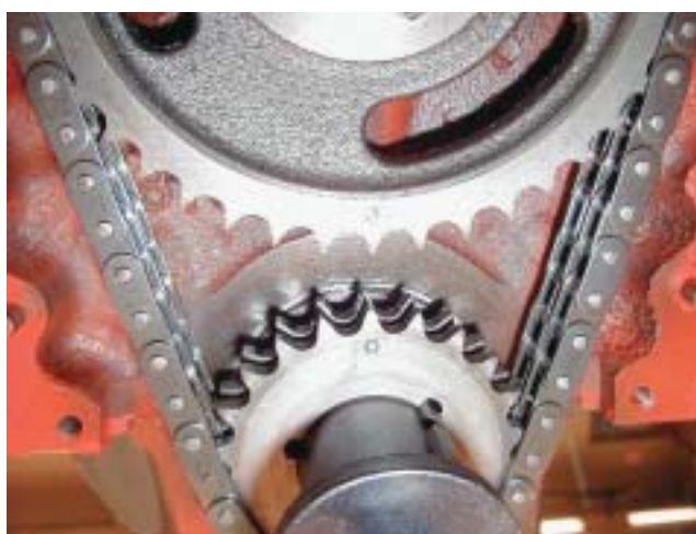
Figure 9–9 A replacement high-performance double roller chain. Even though a bit noisier than a flat-link chain, a roller chain does not stretch as much and will therefore be able to maintain accurate valve timing for a longer time.
