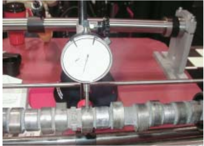
Figure 9-22 A camshaft can be checked for straightness as well as for lift and duration using a dial indicator on a fixture that allows the camshaft to be rotated. This same equipment can be used to check crankshafts.
