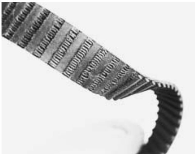
Figure 9-11 Broken timing belt. Also notice the missing teeth. This belt broke at 142 000 km (88 000 mi) because the owner failed to replace it at the recommended interval of 96 000 km (60 000 mi).
