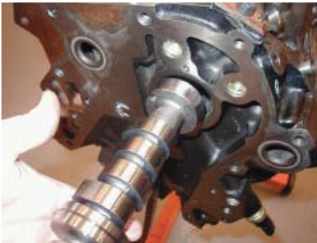
Figure 9-27 Care should be taken when installing a camshaft not to nick or scrape the cam bearings.
