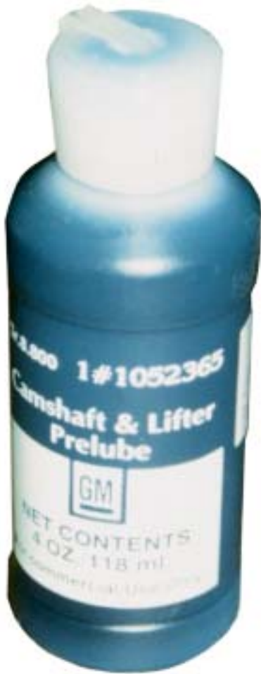
Figure 9-26 Special lubricant such as this one from General Motors is required to be used on the the lobes of the camshaft and the bottom of the flat-bottomed lifters.
