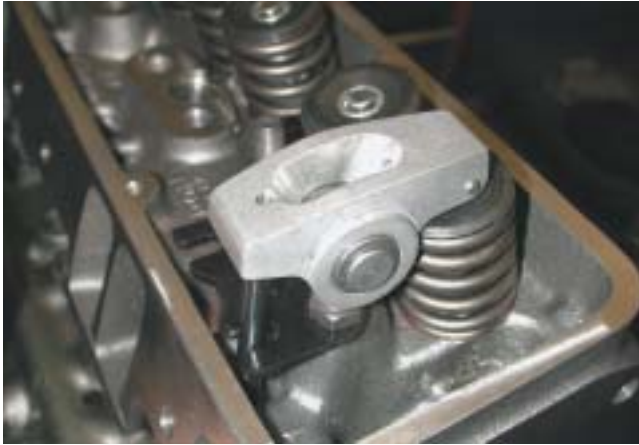
Figure 9-15 A high-performance aluminum roller arm. Both the pivot and the tip that contacts the stem of the valve are equipped with rollers to help reduce friction for more power and better fuel economy.
