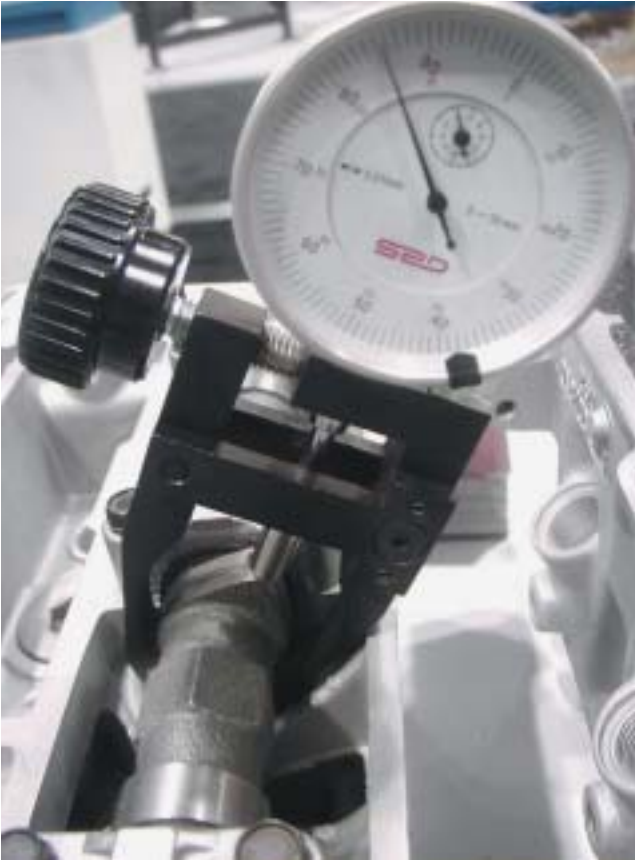
Figure 9-23 The lift of a camshaft lobe can be quickly determined by using this dial indicator that attaches directly to the camshaft.
