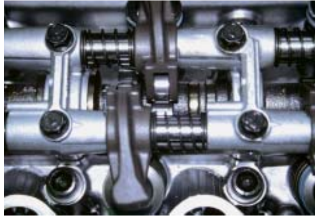
Figure 9–18 Some engines today use rocker shafts to support rocker arms such as the V-6 engine with a single overhead camshaft located in the centre of the cylinder head. This engine uses a roller on the rocker arm.
