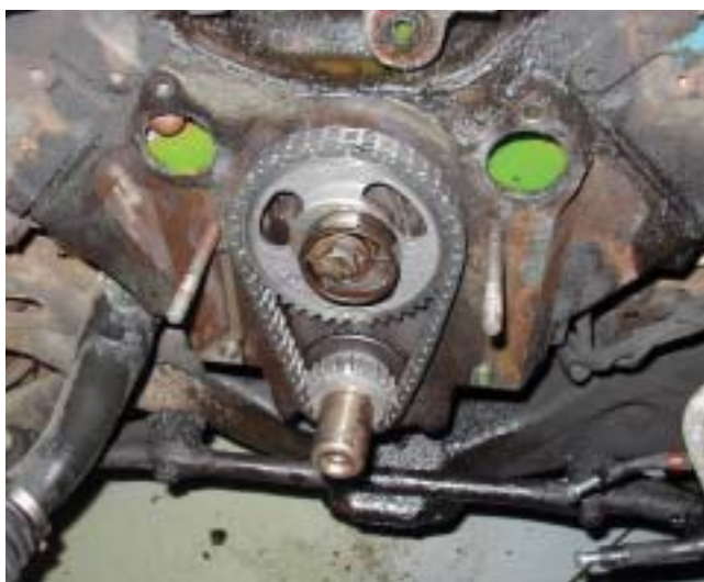
Figure 9–7 A replacement silent chain and sprockets. The original camshaft sprocket was aluminum with nylon teeth to help control noise. This replacement set will not be noticeably louder than the original and should give the owner many thousands of kilometres of useful service.
