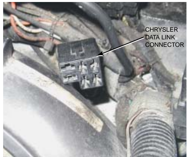
Figure 31–18 An underhood Chrysler data link connector used from 1981 until 1995 on OBD I vehicles.
