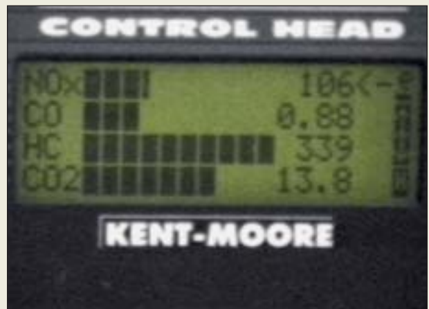
P23-10 This display shows a typical engine at idle after a cold start. Notice the higher-than-normal HC reading.
