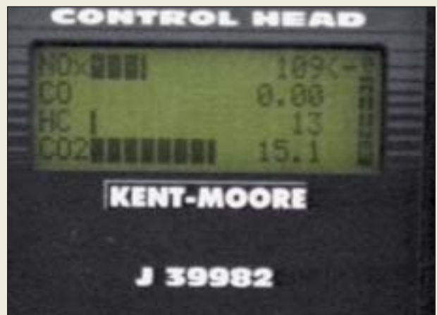
P23-12 After the engine has reached operating temperature, the HC readings are now 13 ppm—well within the normal allowable limit of less than 50 ppm.
