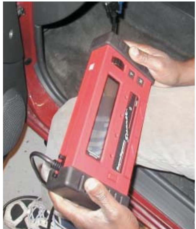
Figure 31-12 Using a Snap-On scan tool to check for engine data that may give an indication as to the root cause of the problem.
