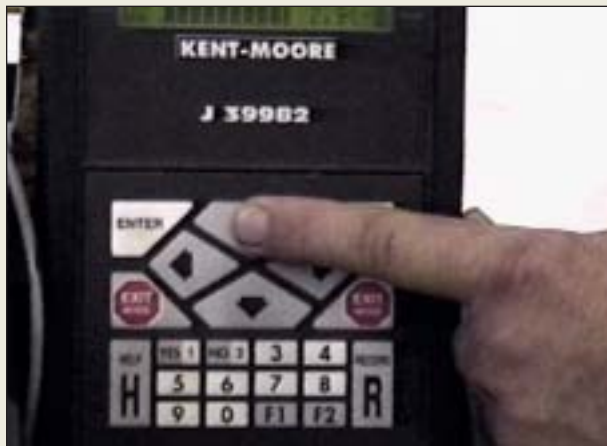
P23-9 Use the up and down arrow keys to scroll up and down the data list to observe the gases. This unit can only display four of the five gases at a time. Because we are not concerned with NO x until the vehicle is driven, this technician selected this display showing CO, HC, CO 2 and O 2 .
