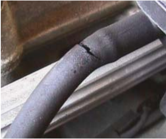
Figure 31-4 All vacuum hoses should be checked to see if they are cracked, swollen, or split.
