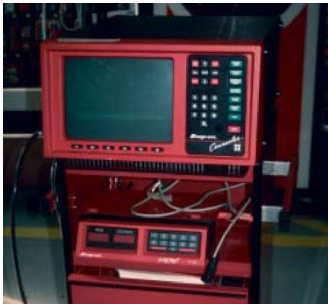
Figure 31-13 An engine analyzer can also be used to help narrow the problem to a particular cylinder or system.
