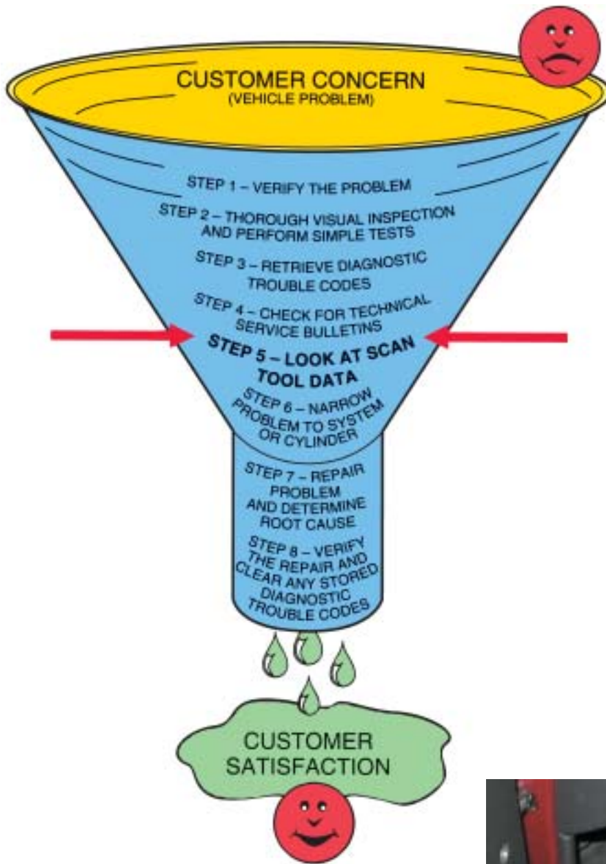
Figure 31-11 Scan tool data is a powerful tool to use to find engine performance malfunctions.
