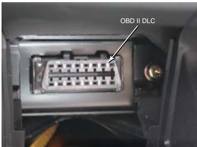
Figure 31–21 An OBD II data link connector (DLC). It is located under the dash and could be covered by a snap-in cover such as on this Acura TL.
