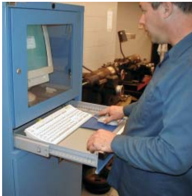
Figure 31–10 After checking for stored diagnostic trouble codes (DTCs), the technician checks to see if there are any technical service bulletins (TSBs) that relate to the vehicle being serviced.
