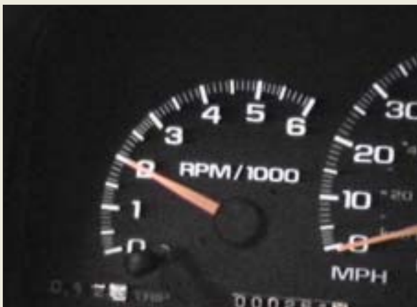
P23-11 To help get the engine, oxygen sensor, and catalytic converter up to operating temperature, operate the engine at 2000 rpm for several minutes.
