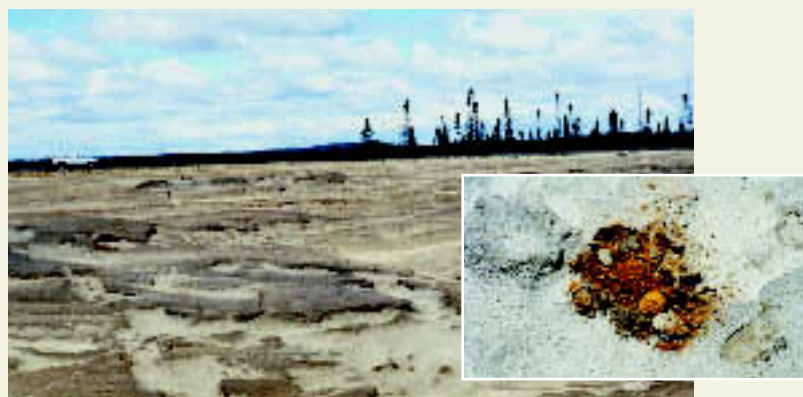
◆ Figure 21.B Metal mine tailings, which appear benign at first glance were revealed to be highly oxidized immediately below the surface (inset). This zone of oxidation extended approximately 40 centimetres down into the tailing. (Photos by Gordon Southam)
