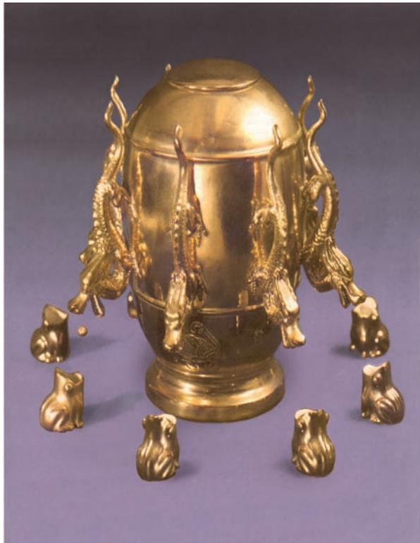
◆ **Figure 10.5** Ancient Chinese seismograph. During an Earth tremor, the dragons located in the direction of the main vibrations would each drop a ball into the mouth of the frog below it. (Photo by James E. Patterson)
