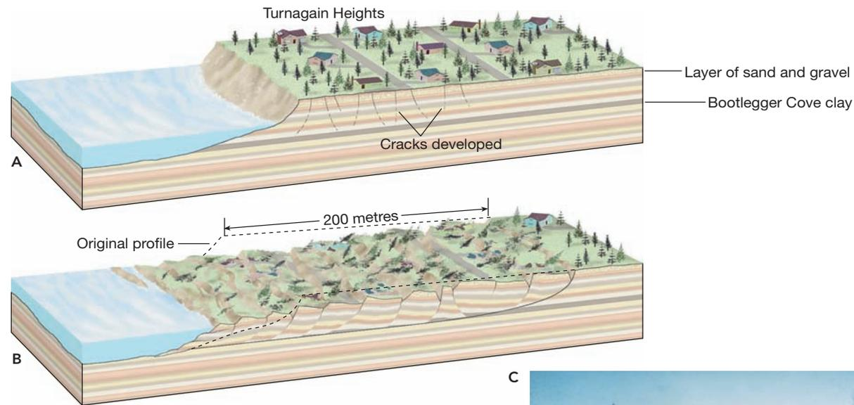
◆ **Figure 10.19** Turnagain Heights slide caused by the 1964 Alaskan earthquake. **A.** Vibrations from the earthquake caused cracks to appear near the edge of the bluff. **B.** Within seconds blocks of land began to slide toward the sea on a weak layer of clay. In less than five minutes, as much as 200 metres of the Turnagain Heights bluff area had been destroyed. **C.** Photo of a small portion of the Turnagain Heights slide. (Photo **C** courtesy of U.S. Geological Survey)
