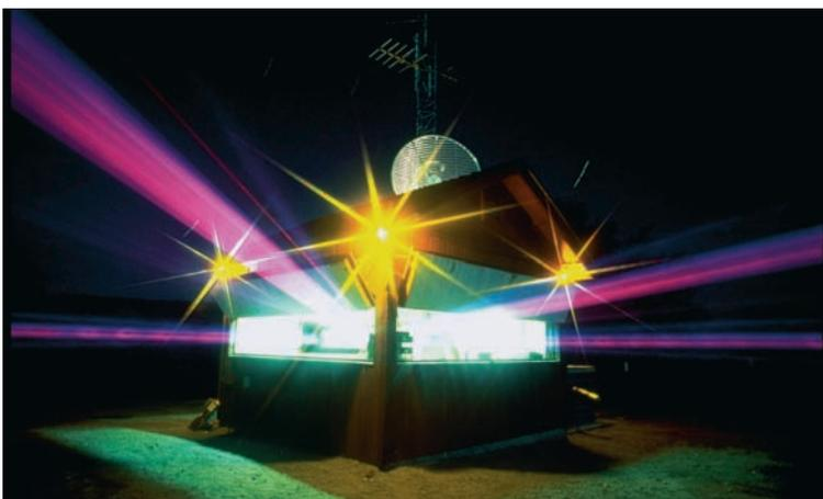
◆ **Figure 10.20** Lasers used to measure movement along the San Andreas Fault. (Photo by John K. Nakata/U.S. Geological Survey)
