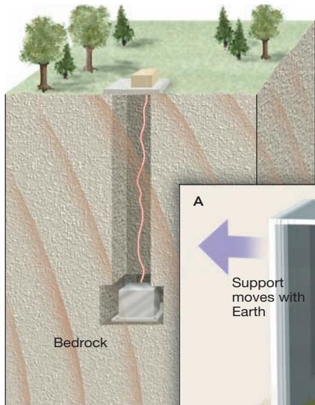
◆ **Figure 10.6** Principle of the seismograph. The inertia of the suspended mass tends to keep it motionless, while the recording drum, which is anchored to bedrock, vibrates in response to seismic waves. Thus the stationary mass provides a reference point from which to measure the amount of displacement occurring as the seismic wave passes through the ground. **A.** Seismograph designed to record horizontal movement. **B.** Seismograph designed to record vertical ground motion.
